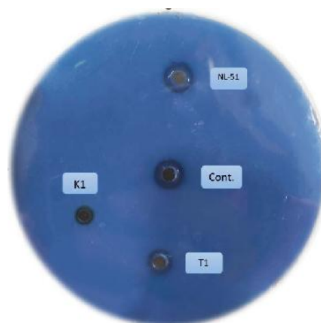
Fig. 1 Determination of inhibitors of proteolytic enzymes in research samples by gel diffusion method.
